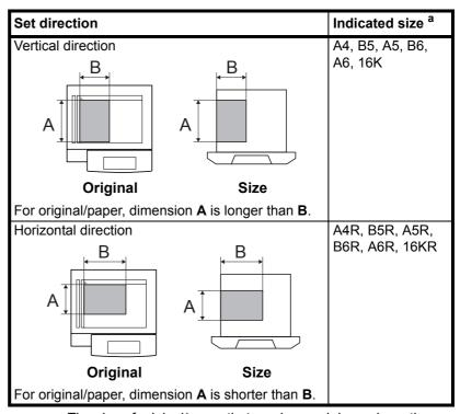
a. The size of original/paper that can be used depends on the function and source tray. For further details, refer to the page detailing that function or source tray.
